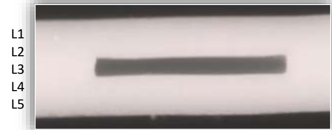
Shrinkage ratio in Z direction: ~50%
