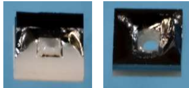
two exemplary fracture pattern (left: fracture at bondinterface, right: bulk material fracture) [3]
