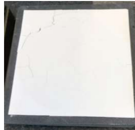
SiCer substrate with loose relesetape on both sides
