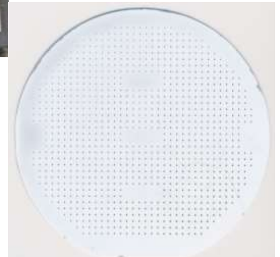
Final SiCer substrate after cleaning process
